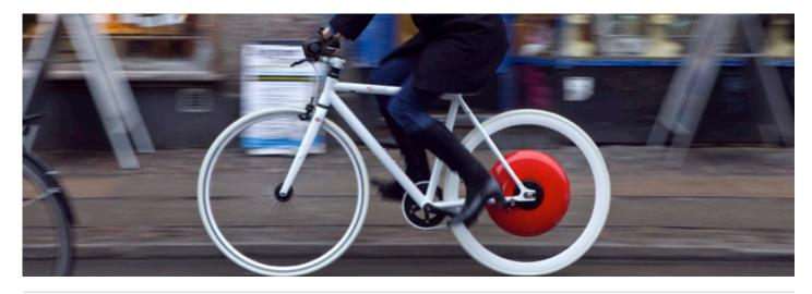
Picture 4. The Copenhagen Wheel transforms your bicycle into a smart electric hybrid. The Wheel contains a motor, batteries, multiple sensors, wireless connectivity and an embedded control system. The Wheel learns how you pedal and integrates seamlessly with your motion, multiplying your pedal power.
